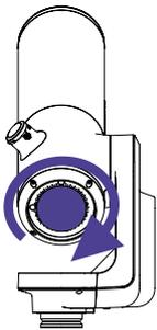
On your smartphone or tablet screen, adjust the focus of the eVscope/ eQuinox by turning the focus wheel located at the base of the instrument until the image is clear.
